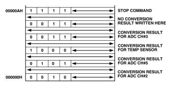
Figure 12. Typical External Memory Configuration Post ADC DMA Operation
